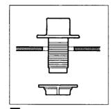
If your faucet has a spray, place hole guide down through hole at extreme right of sink top. Add mounting nut to underside and FINGER tighten firmly.
